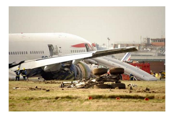
British Airways Flight 38, a Boeing 777-200ER, crash-landed just short of the runway at London Heathrow Airport on January 17, 2003. The investigation revealed that the accident was primarily caused by a fuel flow restriction in the
