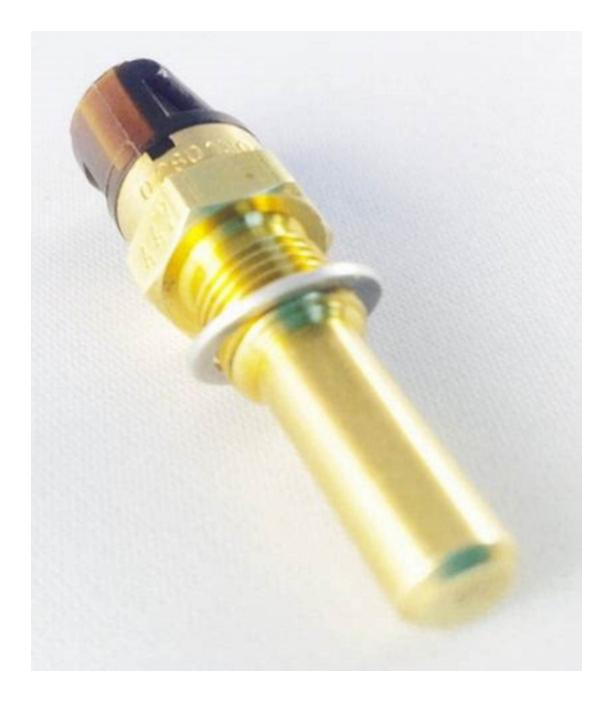
The temperature sensor is usually located near the thermostat housing or on the cylinder head. It consists of a temperature-dependent semiconductor element that changes its resistance based on temperature variations. This change in
