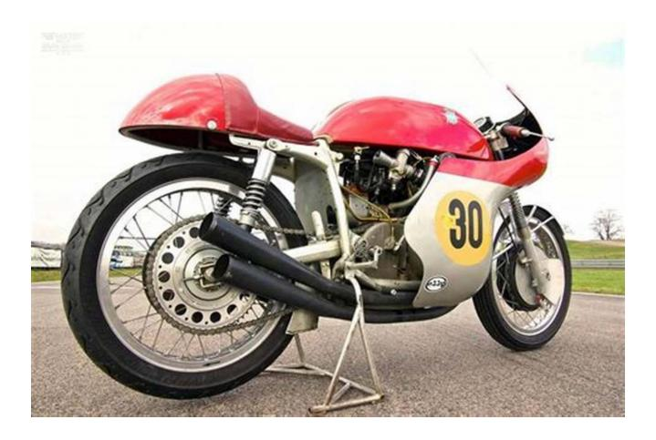
The MV Agusta 500 Grand Prix featured a 498cc four-cylinder engine, producing a staggering 72 horsepower at 12,000rpm. With its lightweight frame and exceptional handling, this motorcycle effortlessly danced through tight corners and blistering straights.
