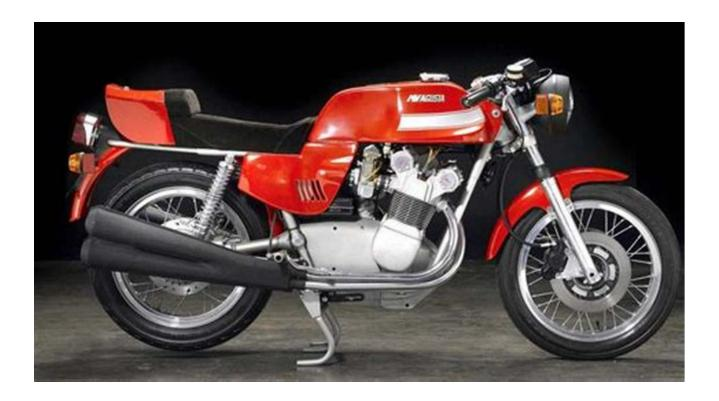
Powering the MV Agusta 750 Sport America was a 789cc four-cylinder engine, delivering an impressive 70 horsepower. With its distinctive red, white, and blue paint scheme, this motorcycle became an unmistakable symbol of Italian craftsmanship and engineering prowess.
